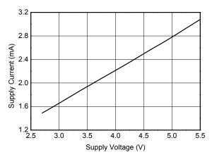
Supply Current vs. Supply Voltage
