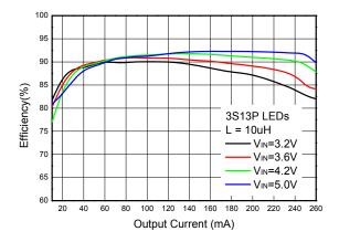
**Efficiency vs. Output Current**
