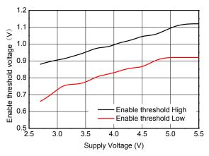
**Enable Threshold Voltage vs. Supply Voltage**
