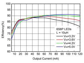
**Efficiency vs. Output Current**
