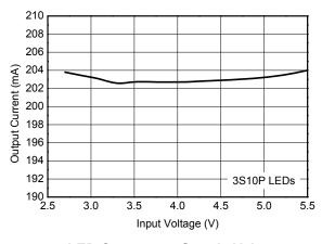
LED Current vs. Supply Voltage
