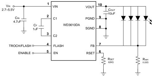
Figure 2. Multiple LED flash circuit @1000mA flash current
