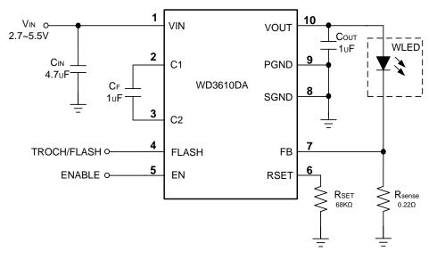
Figure1. Single LED flash circuit @ 850mA flash current
